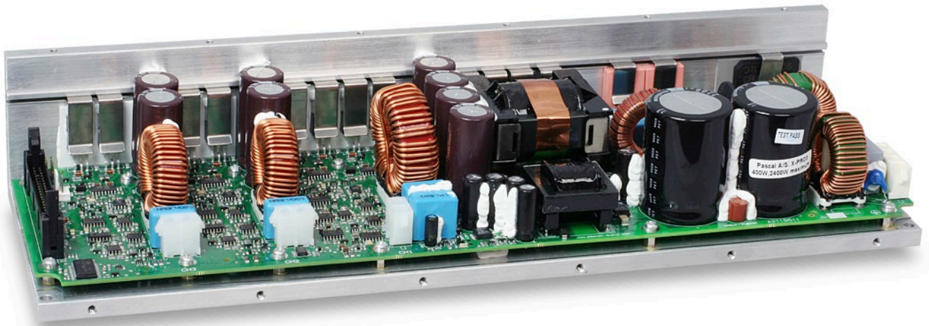
X-PRO3 Power Amplifier Unit with dedicated high power channel and two mid power channels
