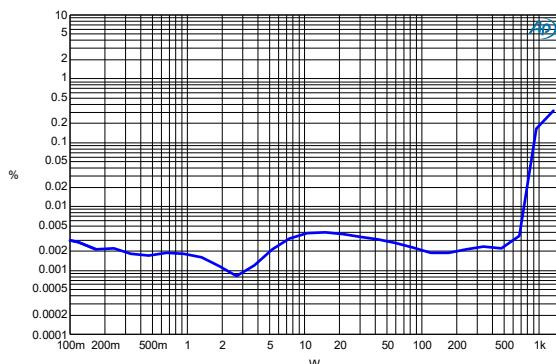
CCIF vs power  $R_L=4$  ohm, channel 1,  $f_1=18\text{kHz}$ ,  $f_2 =19\text{kHz}$
