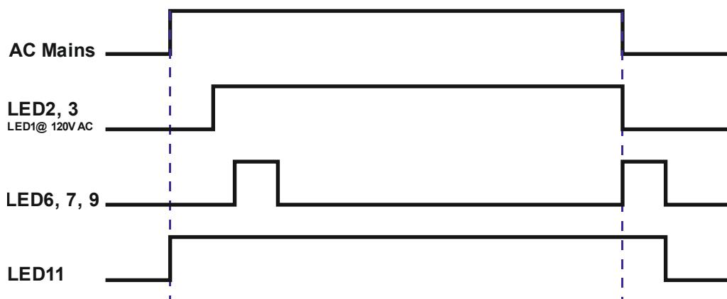
Figure 4-2: LED timing during start-up and shut-down
