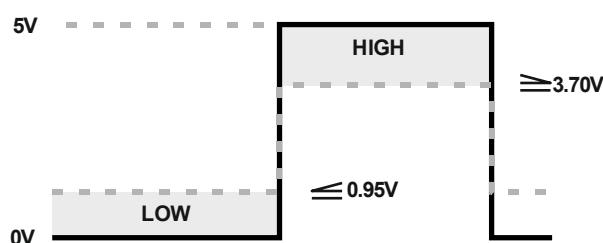
Figure 4-5: High and Low voltage levels for logic input
