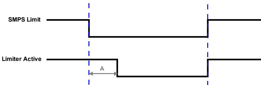
Figure 7-1: SMPS limit, A = Typically 1 sec.
