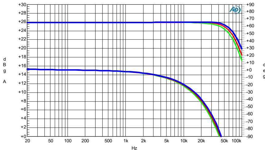
Frequency response,  $4\Omega$  (green),  $8\Omega$  (red) and open load (blue). Top – amplitude. Bottom – phase.
