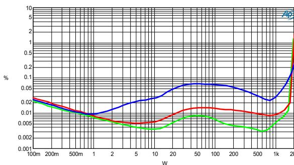
THD+N vs. Po, Channel 1, 100Hz (green), 1kHz (red), 6,67kHz (blue), 4Ω<sup>1</sup>
