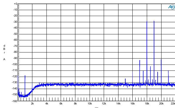
CCIF FFT, Channel 1,  $f_1=18\text{kHz}$ ,  $f_2 =19\text{kHz}$   $R_L=4$  Ohm,  $P_0 =10\text{W}$ .
