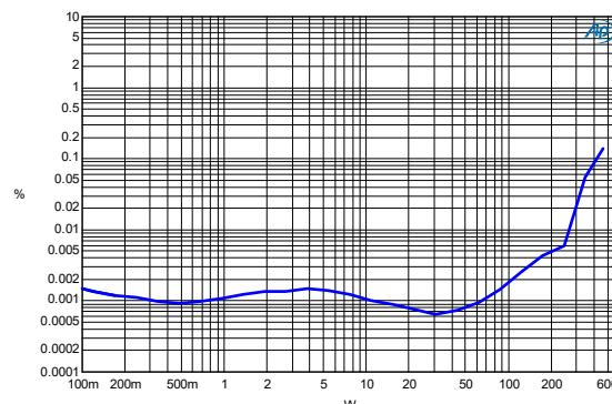
CCIF vs power  $R_L=4$  ohm, channel 2/3,  $f_1=18\text{kHz}$ ,  $f_2 =19\text{kHz}$
