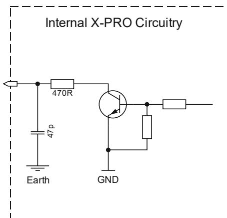
Figure 4-3: Open Collector output
