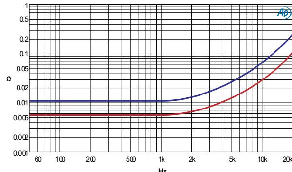
Output impedance, Channel 2/3,  $I_{out}=1A_{RMS}$ ,
