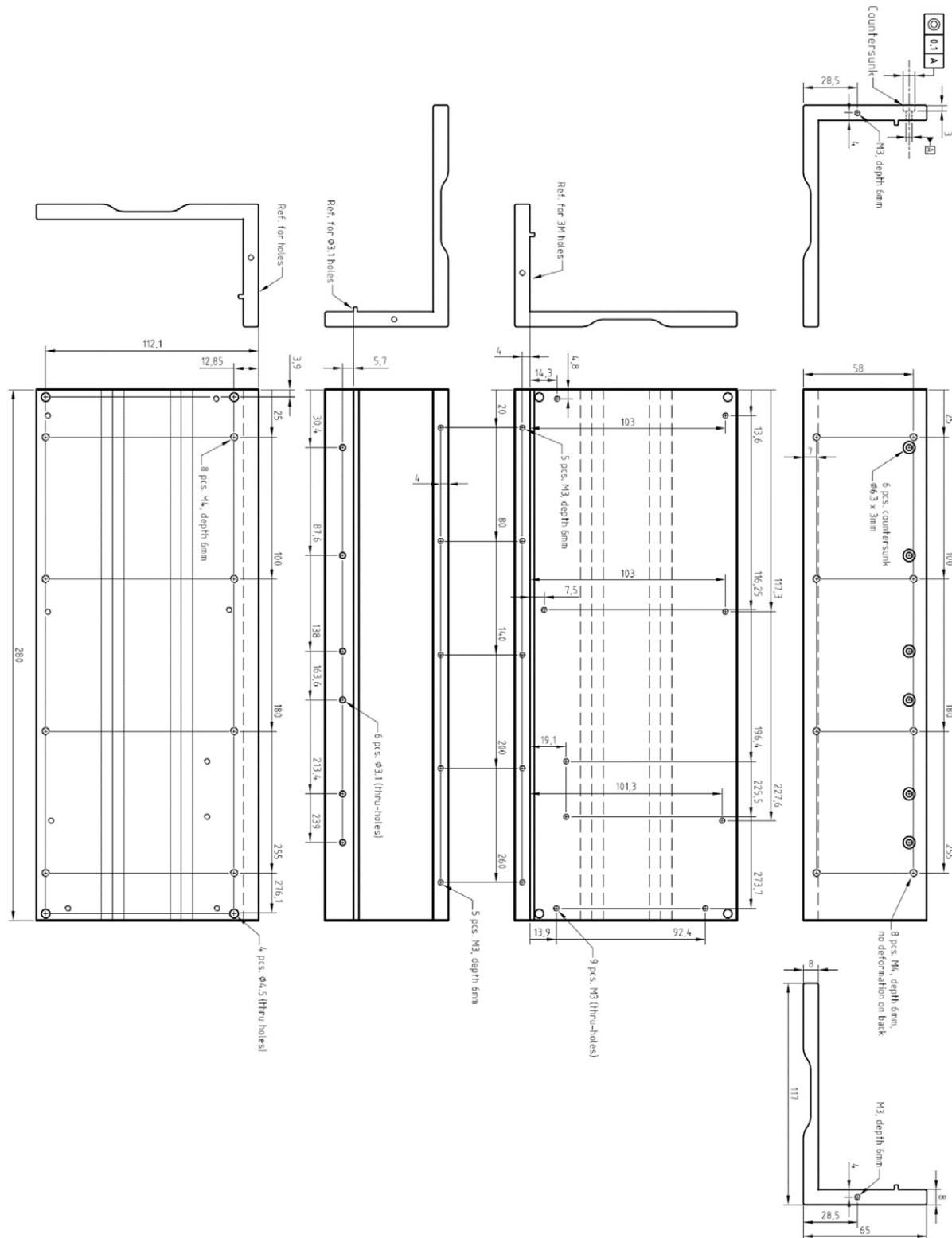
Figure 8-1: Mechanical dimensions of the X-PRO1 heat sink - All dimensions in mm
