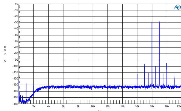
CCIF FFT, Channel 2/3,  $f_1=18\text{kHz}$ ,  $f_2 =19\text{kHz}$   $R_L=4$  Ohm,  $P_0 =10\text{W}$ .
