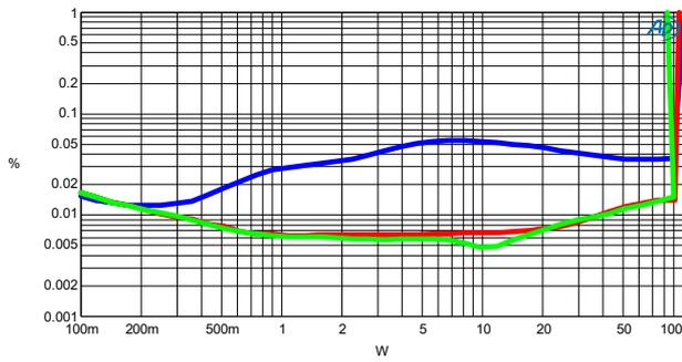
Figure 3-3 THD+N vs. Power @ 4Ω, 230VAC
