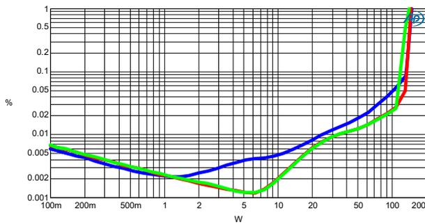
Figure 3-9: THD+N vs. Power@ 40Ω, 120VAC
