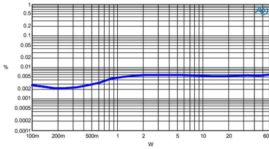
Figure 3-13: CCIF vs. Power -  $R_L=4\Omega$
