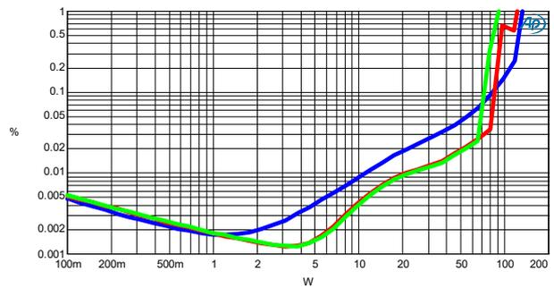
Figure 3-10: THD+N vs. Power @ 66Ω, 120VAC
