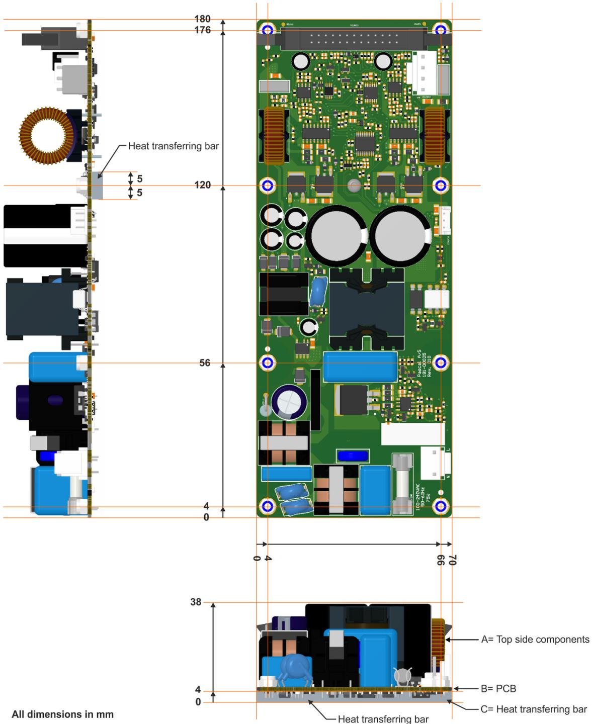
Figure 7-1: Mechanical specifications for the U-PRO2SD module
