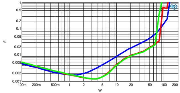
Figure 3-8: THD+N vs. Power @ 66Ω, 230VAC
