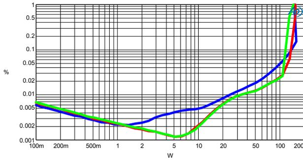
Figure 3-7: THD+N vs. Power@ 40Ω, 230VAC
