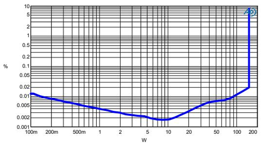
Figure 3-19 TIM vs. Power -  $R_L=40\Omega$ ,  $230V_{AC}$
