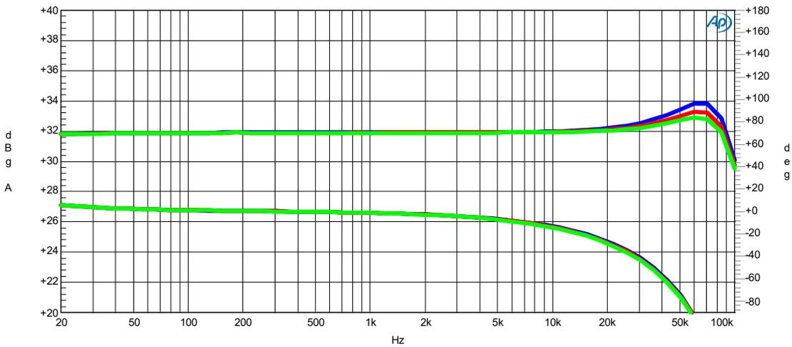
Figure 3-2: Frequency response (op curves: Amplitude, Bottom curves: Phase) 40Ω (green), 66Ω (red) and Open Load (blue)
