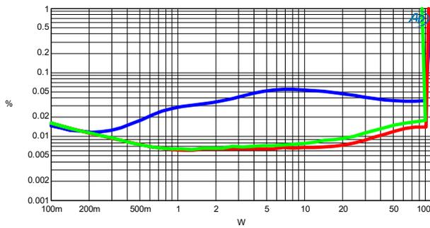
Figure 3-5 THD+N vs. Power @ 4Ω, 120VAC
