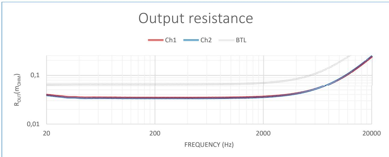
Figure 3-21: Output resistance - Measurement made at the mating part of the output connector. Connector resistance thereby included. Ch1 (red), Ch2 (blue), Ch1+Ch2 (grey)
