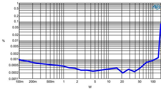
Figure 3-17 CCIF vs. Power -  $R_L=40\Omega$
