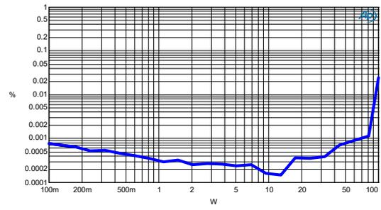
Figure 3-18 CCIF vs. Power -  $R_L=66\Omega$
