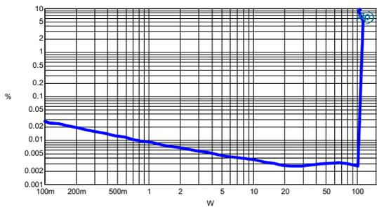
Figure 3-15: TIM vs. Power -  $R_L=4\Omega$ ,  $230V_{AC}$  Ch1 (blue)
