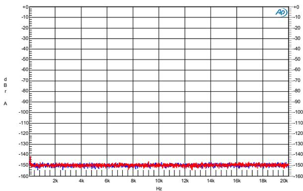
Figure 3-11: FFT idle - 8Ω SE
