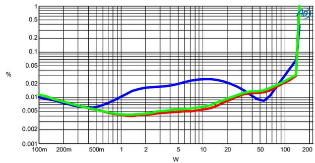
Figure 3-6 THD+N vs. Power @ 8Ω, 120VAC
