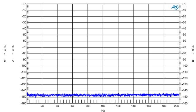
Figure 3-12: FFT idle - 66Ω BTL
