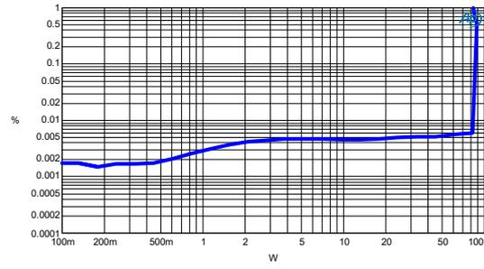
Figure 3-14: CCIF vs. Power -  $R_L=8\Omega$
