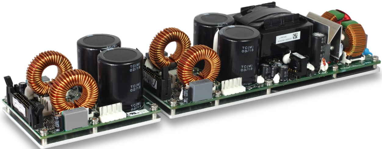
L-PRO2S + L-A2 800 + 800 + 800 + 800 W Lo-Z 1500 + 1500 W Hi-Z direct drive
