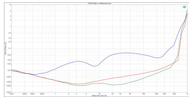
Figure 3-6: THD+N vs. Power @4Ω CH2, 230VAC/120VAC
