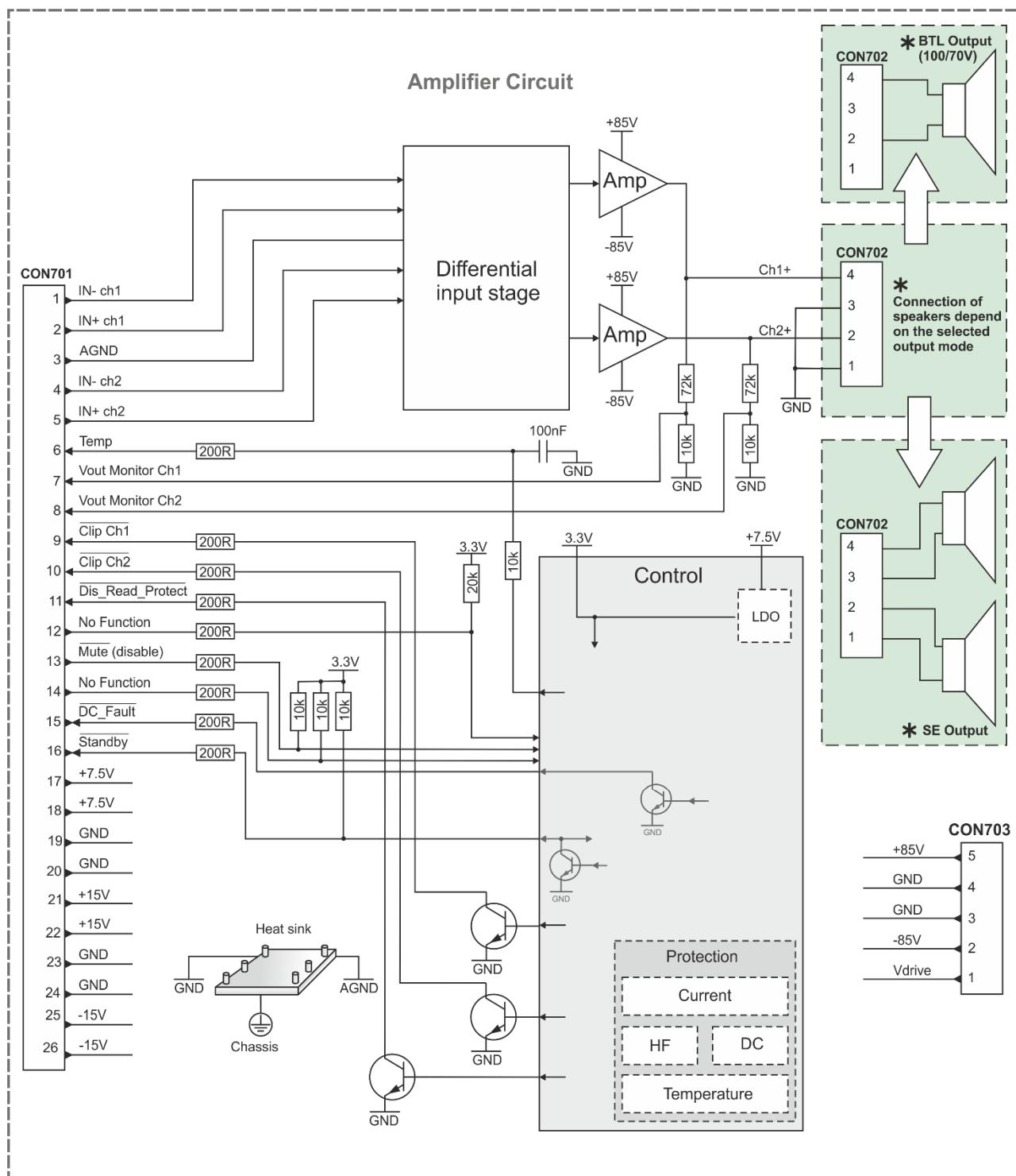
Figure 5-1: Block diagram showing L-A2 module functionality.
