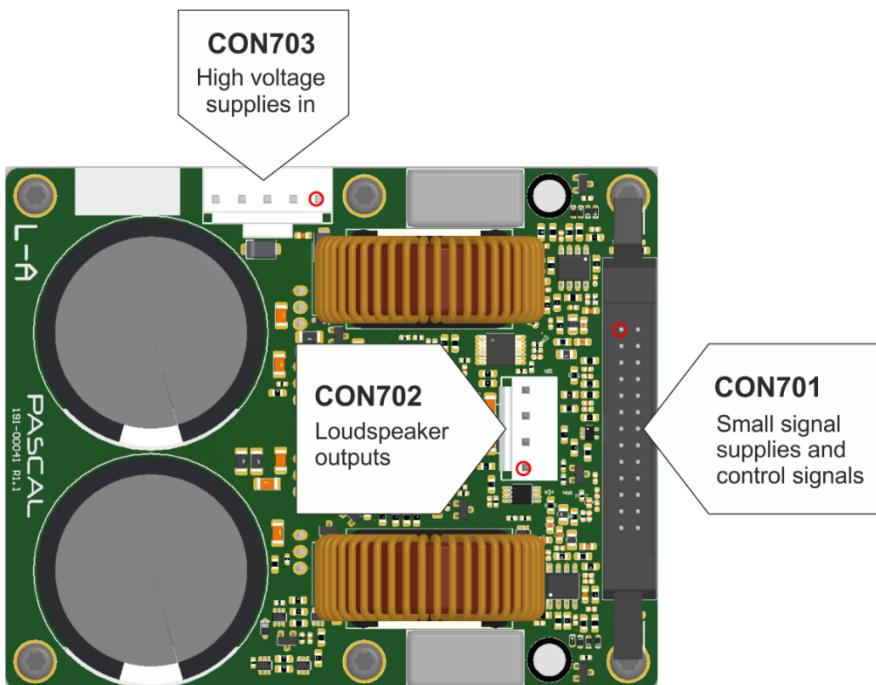
Figure 6-1: L-A2 extension amplifier module connectors - red circle indicates pin 1
