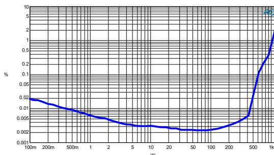
Figure 3-15: TIM vs. Power -  $R_L=4\Omega$
