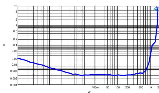
Figure 3-20 TIM vs. Power -  $R_L=6.67\Omega$
