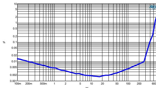
Figure 3-16: TIM vs. Power -  $R_L=8\Omega$
