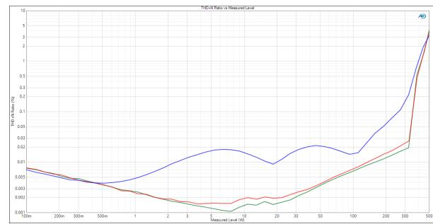
Figure 3-4: THD+N vs. Power @8Ω CH2, 230VAC/120VAC
