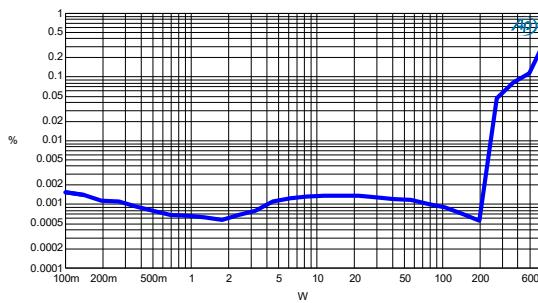
Figure 3-13: CCIF vs. Power -  $R_L=4\Omega$
