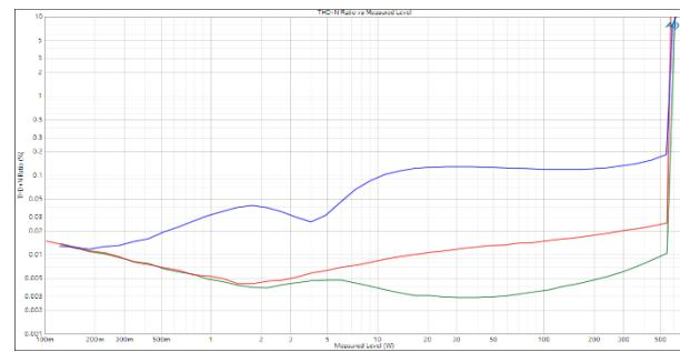
Figure 3-8: THD+N vs. Power @2Ω CH2, 230VAC/120VAC
