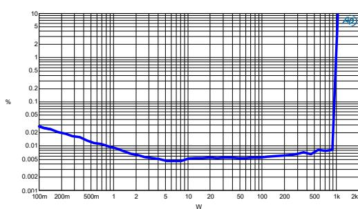
Figure 3-19 TIM vs. Power -  $R_L=4\Omega$
