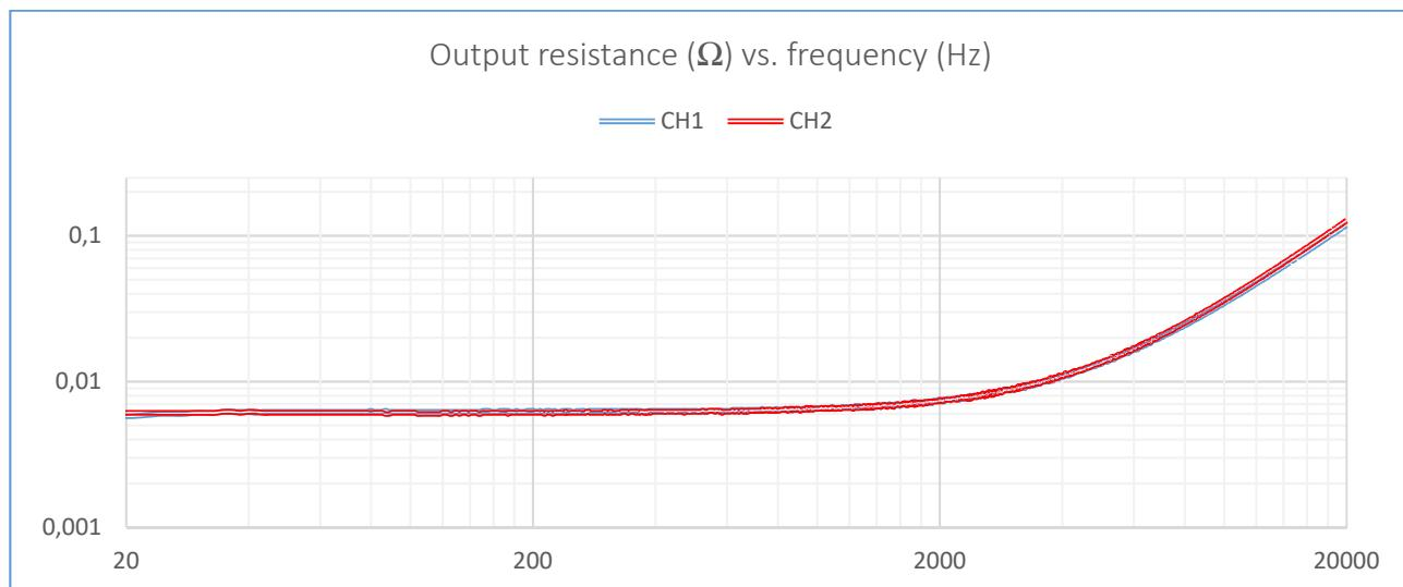
Figure 3-21: Output resistance<sup>1</sup> - Measurement made at the mating part of the output connector. Connector resistance thereby included.
