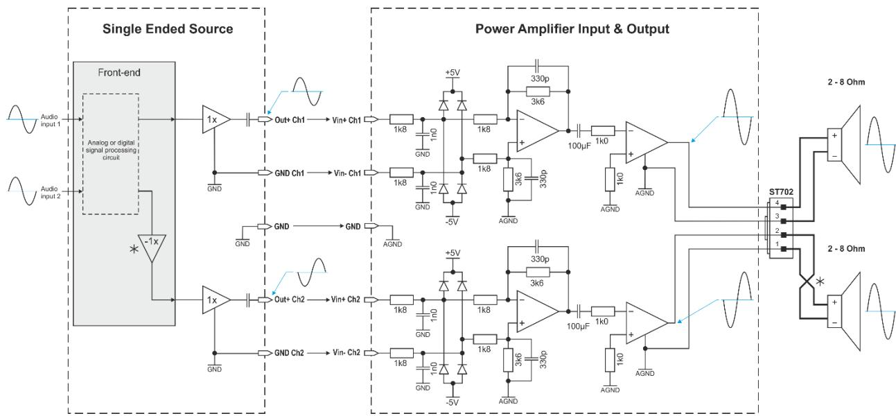
Figure 5-2: L-A2 extension amplifier module shown in Single Ended (SE) output configuration for 2 – 8 Ohm applications.
