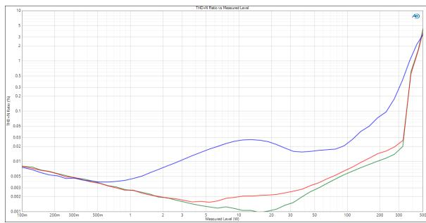
Figure 3-3: THD+N vs. Power @8Ω CH1, 230VAC/120VAC
