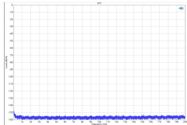
Figure 3-12: FFT idle - (BTL)  $6.67\Omega$
