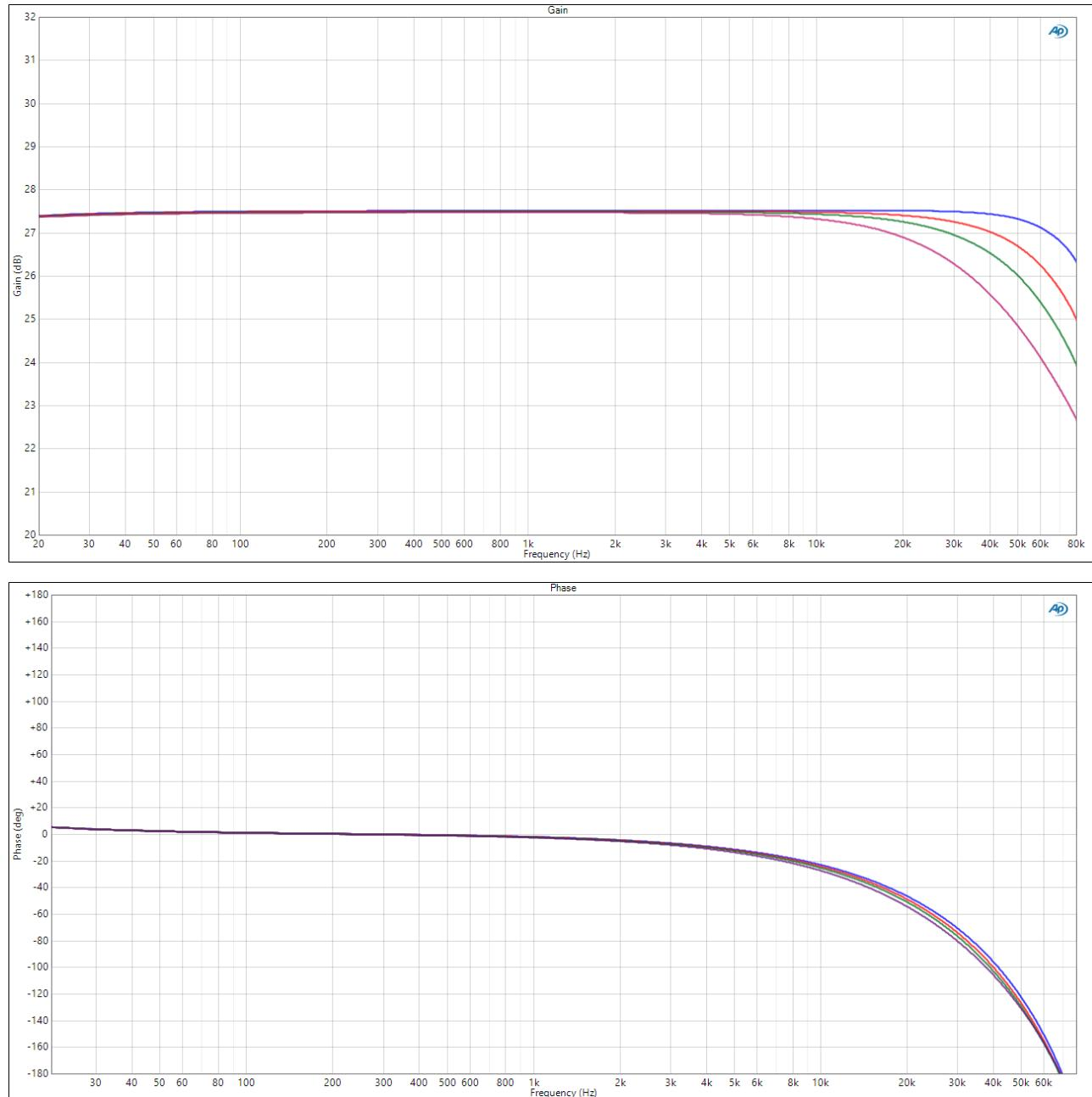
Figure 3-1: Frequency response (Top curves: Amplitude, Bottom curves: Phase)
