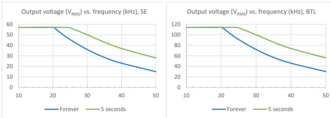
Figure 3-24: Max  $V_{out}$  vs. frequency vs. time (SE mode)
