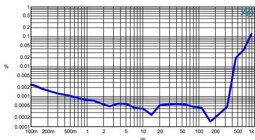
Figure 3-17 CCIF vs. Power -  $R_L=4\Omega$
