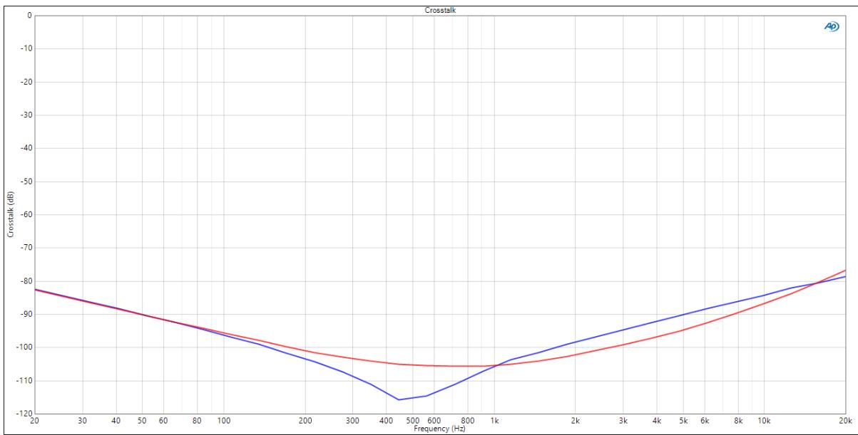
Figure 3-23: Cross talk - Ch.1 @ Po,ch2=50W 8Ω (blue), Ch.2 @ Po,ch1=50W 8Ω (red)
