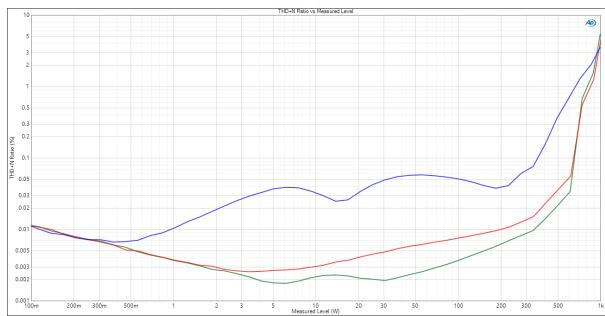
Figure 3-5: THD+N vs. Power @4Ω CH1, 230VAC/120VAC
