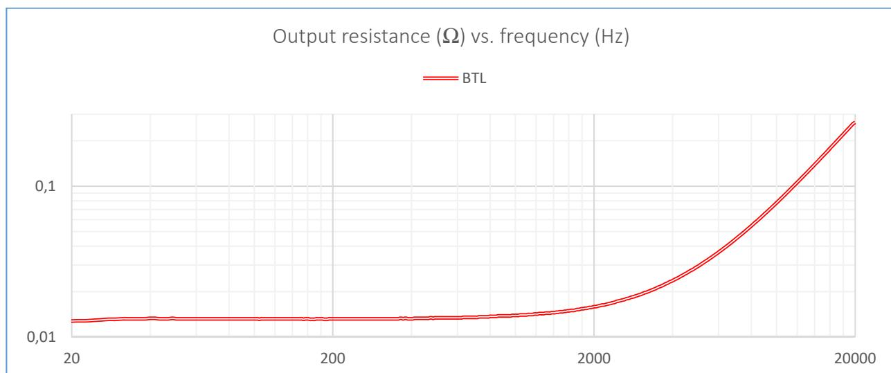
Figure 3-22: Output resistance<sup>1</sup> - Measurement made at the mating part of the output connector. Connector resistance thereby included.
