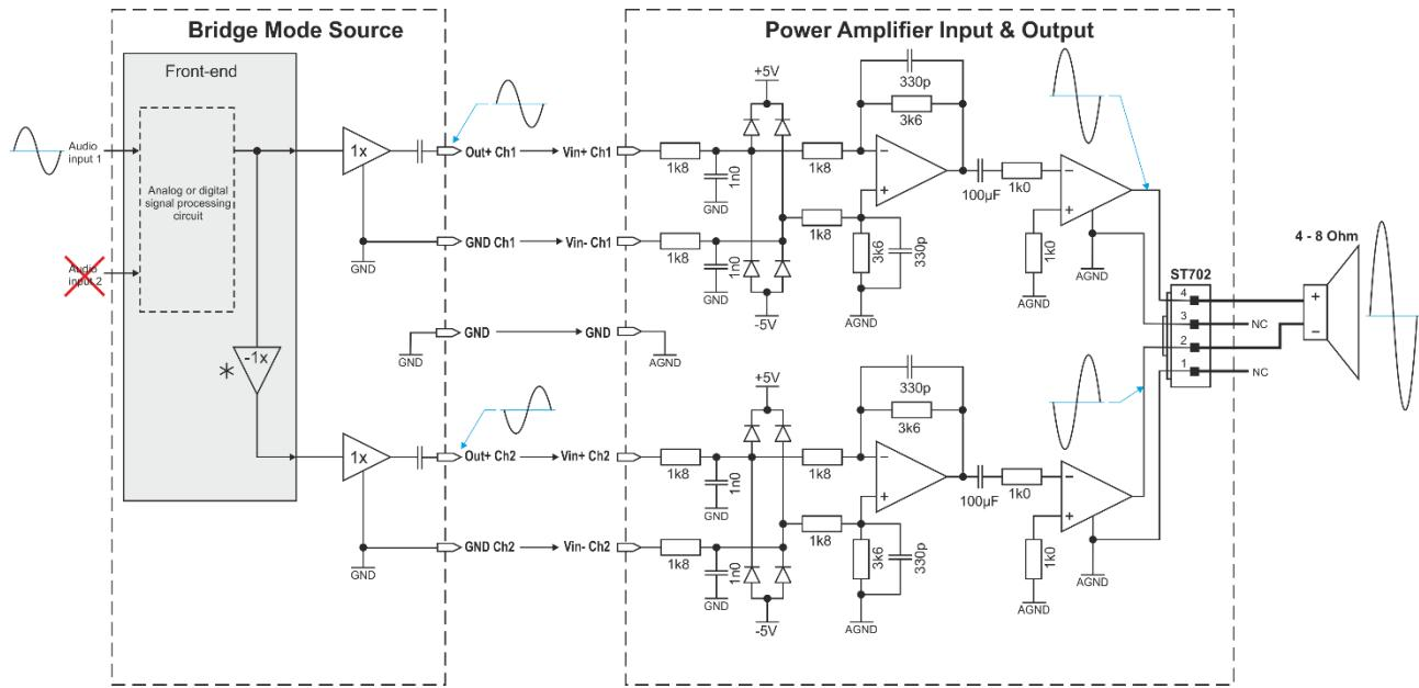
Figure 5-3: L-A2 extension amplifier module shown in Bridge Tied Load (BTL) output configuration for 4 - 8 Ohm applications.
