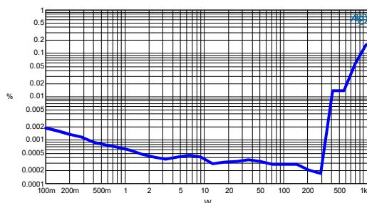
Figure 3-18 CCIF vs. Power -  $R_L=6.67\Omega$
