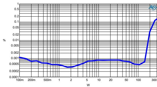
Figure 3-14: CCIF vs. Power -  $R_L=8\Omega$
