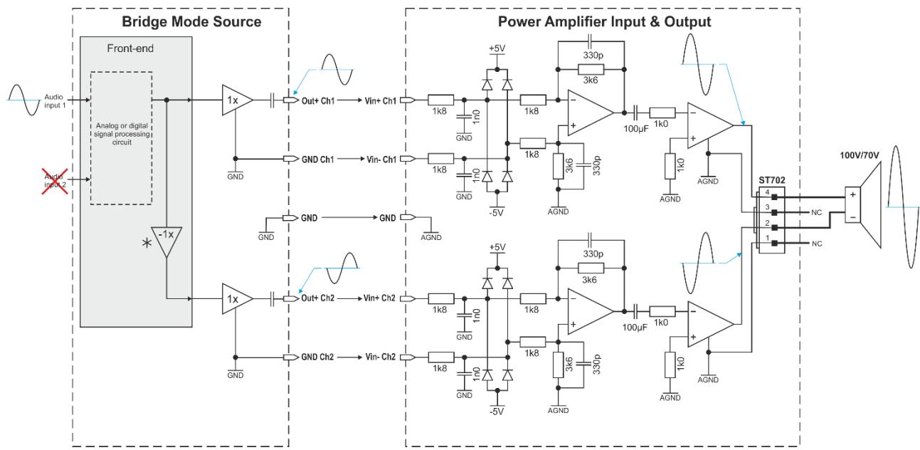
Figure 5-4: L-A2 extension amplifier module shown in Bridge Tied Load (BTL) output configuration for 100/70V applications.
