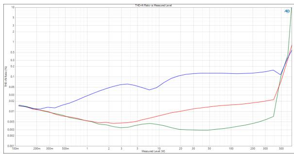
Figure 3-7: THD+N vs. Power @2Ω CH1, 230VAC/120VAC
