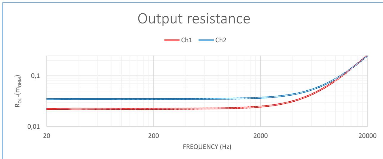
Figure 3-21: Output resistance<sup>1</sup> – Measurement made at the mating part of the output connector. Connector resistance thereby included. Ch1(LF) (red), Ch2(HF) (blue)
