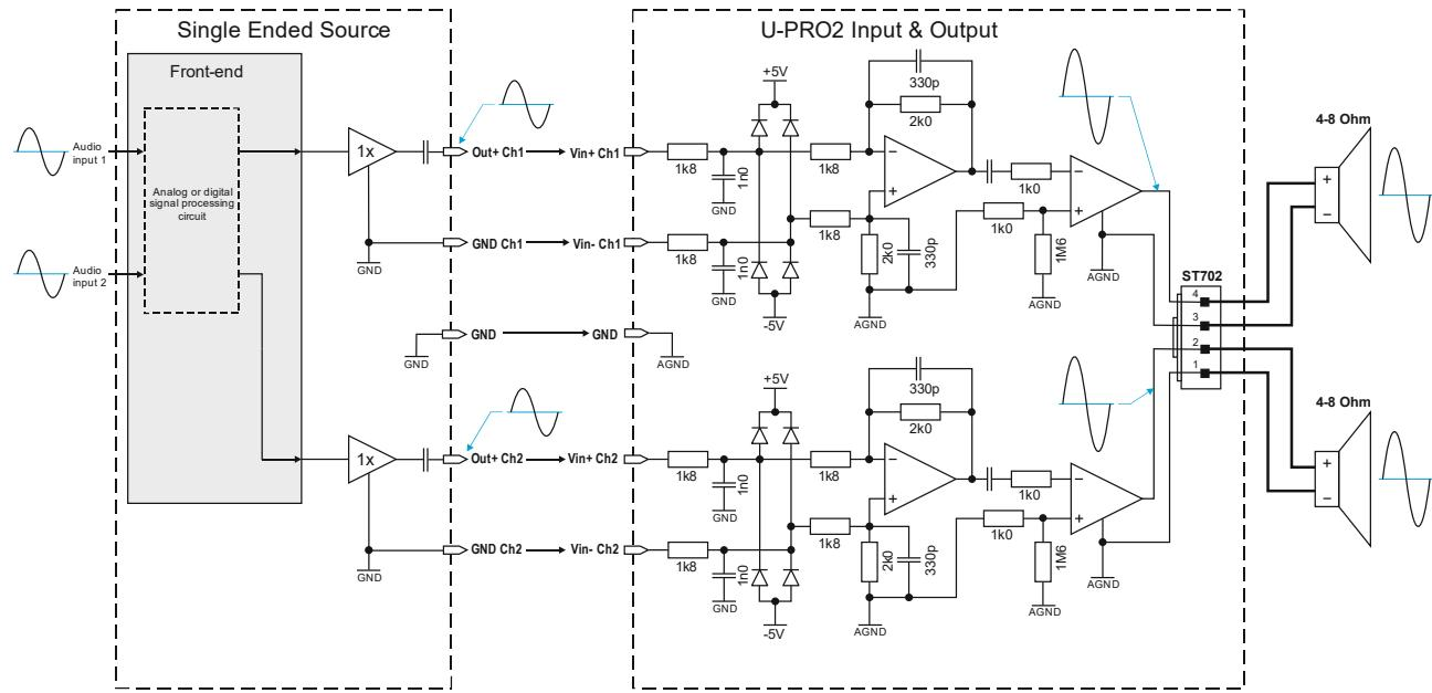
Figure 5-2: U-PRO2 Amplifier module with Single Ended (SE) outputs connected to woofer (LF) and tweeter (HF)
