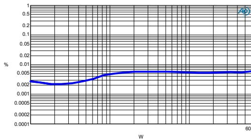
Figure 3-17 CCIF vs. Power -  $R_L=4\Omega$
