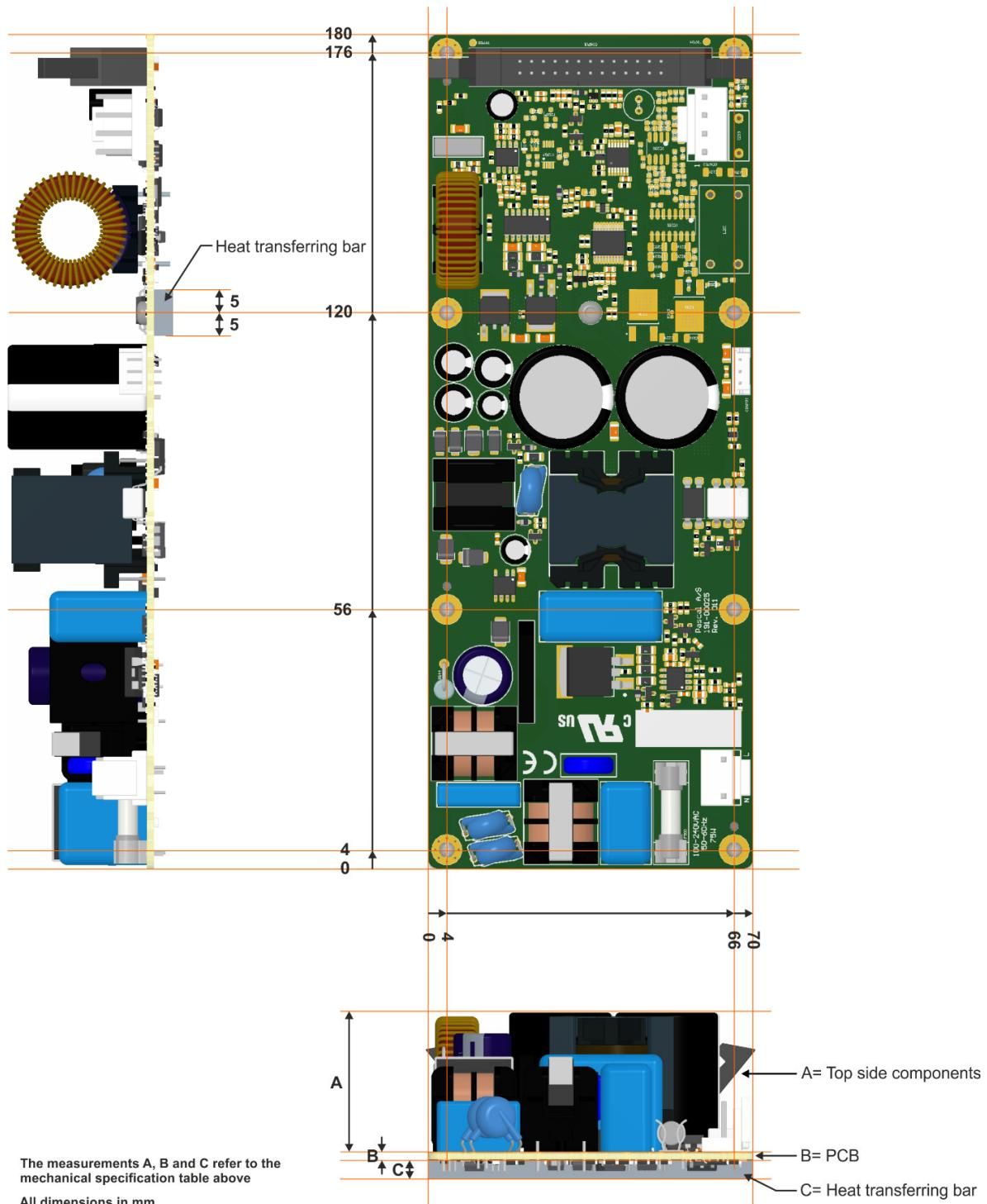
Figure 7-1: Mechanical outline and specifications for the U-PRO1 module
