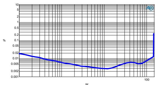
Figure 3-20 TIM vs. Power -  $R_L=8\Omega$
