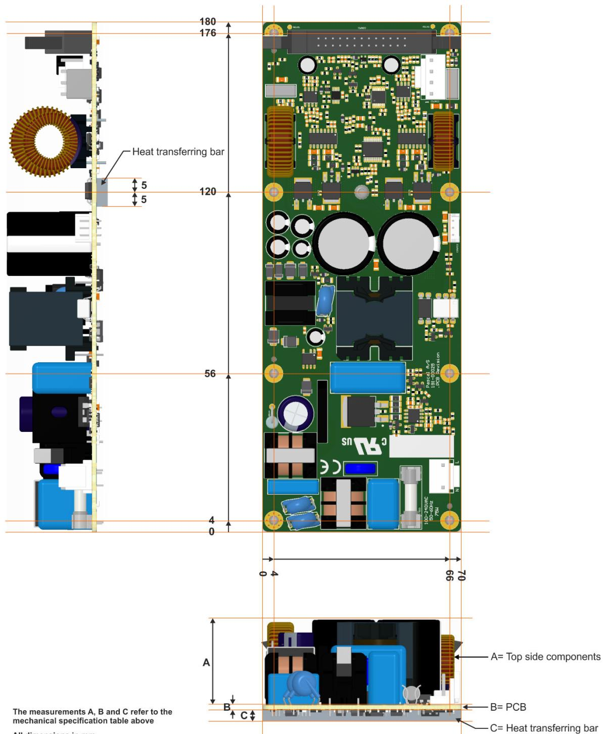
Figure 7-2: Mechanical specifications for U-PRO2 module
