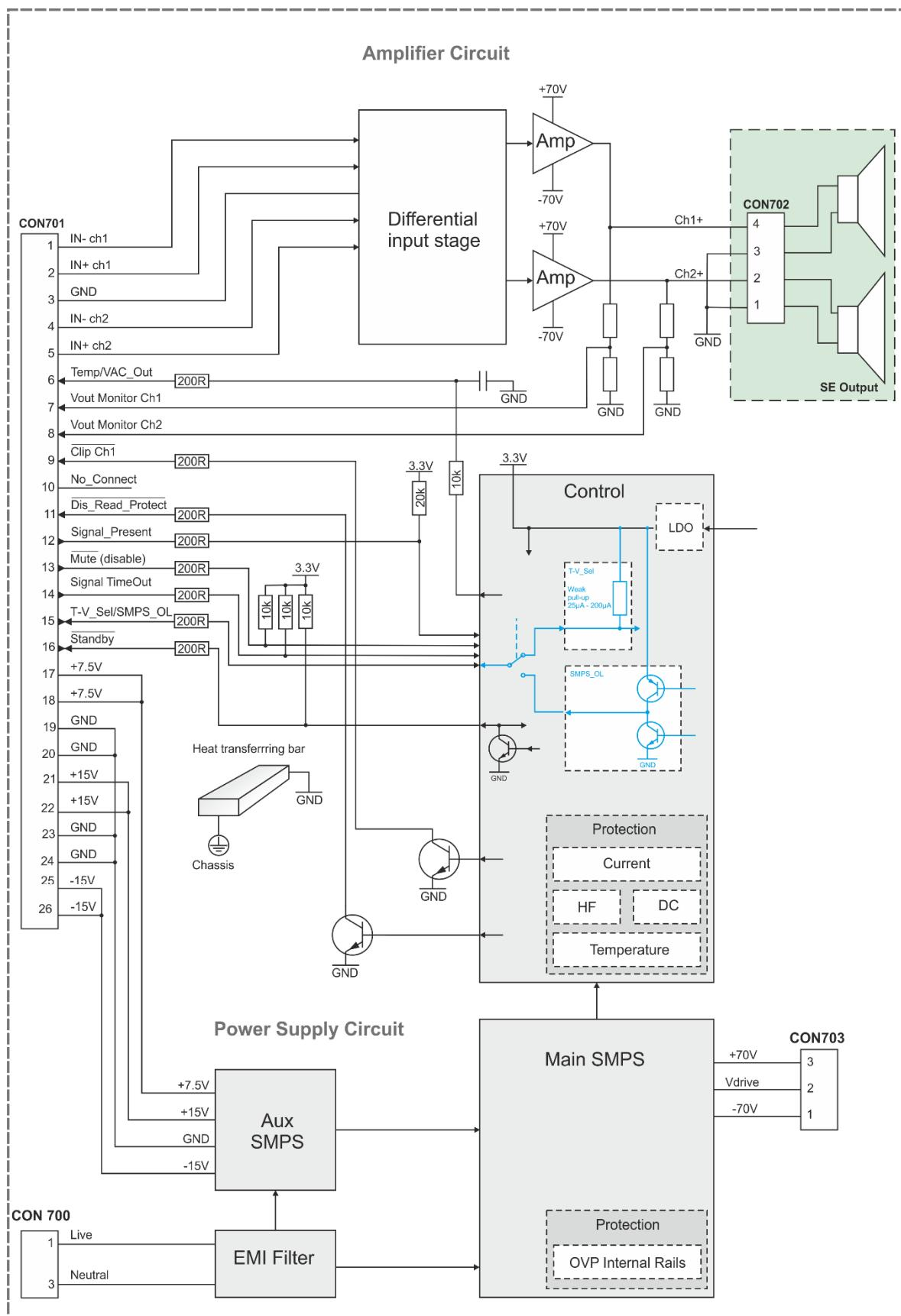
Figure 5-1: Block diagram showing U-PRO2 module functionality. For U-PRO: Channel 2 circuitry is eliminated
