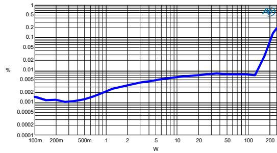
Figure 3-14: CCIF vs. Power -  $R_L=8\Omega$
