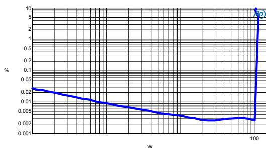
Figure 3-19 TIM vs. Power -  $R_L=4\Omega$
