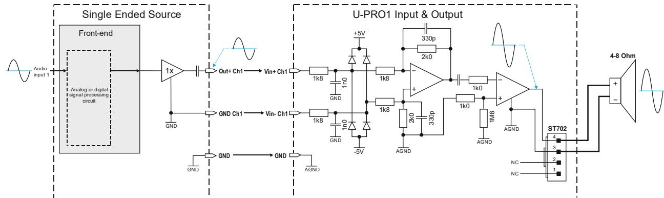
Figure 5-3: U-PRO1 Amplifier module with Single Ended (SE) output connected to a subwoofer (LF)
