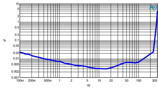
Figure 3-16: TIM vs. Power -  $R_L=8\Omega$
