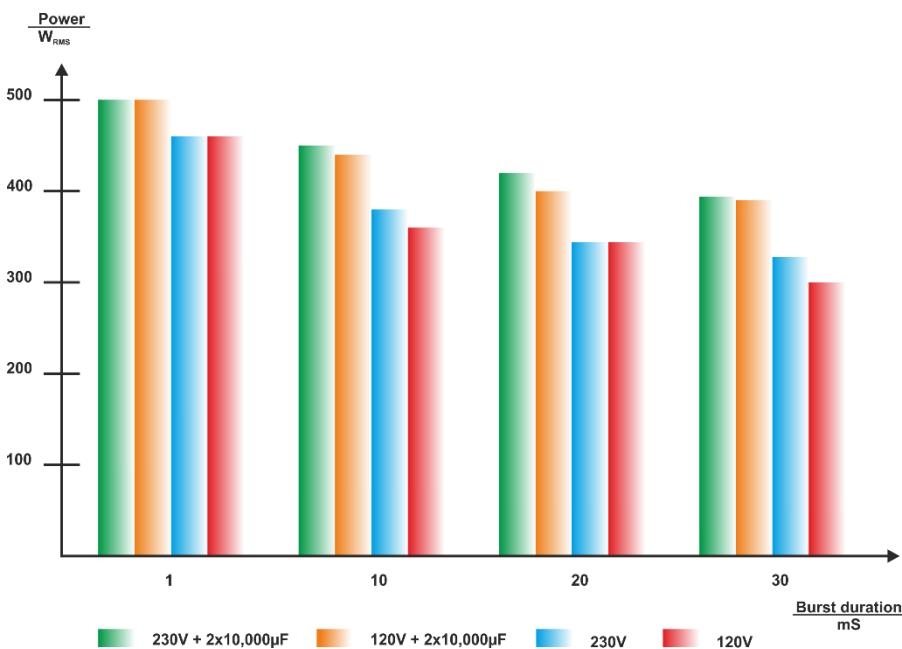
Figure 3-7: Burst power Ch1 (LF) @ 4Ω, 1kHz
