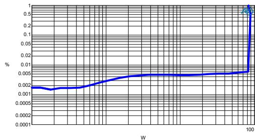
Figure 3-18 CCIF vs. Power -  $R_L=8\Omega$
