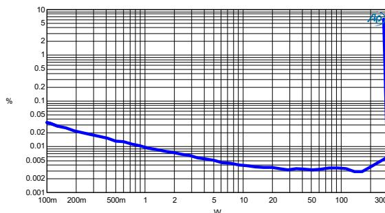
Figure 3-15: TIM vs. Power -  $R_L=4\Omega$
