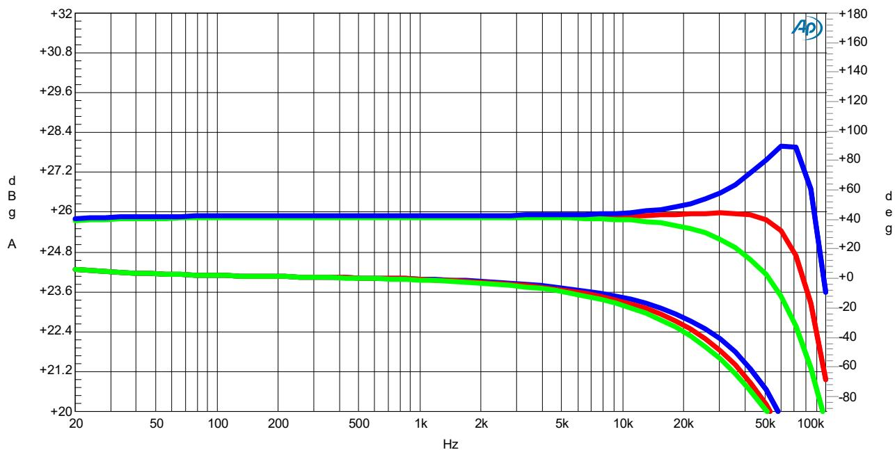
Figure 3-2: Frequency response (op curves: Amplitude, Bottom curves: Phase)
