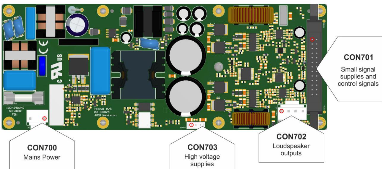
Figure 6-2: U-PRO2 Amplifier module connectors - red circle indicates pin 1
