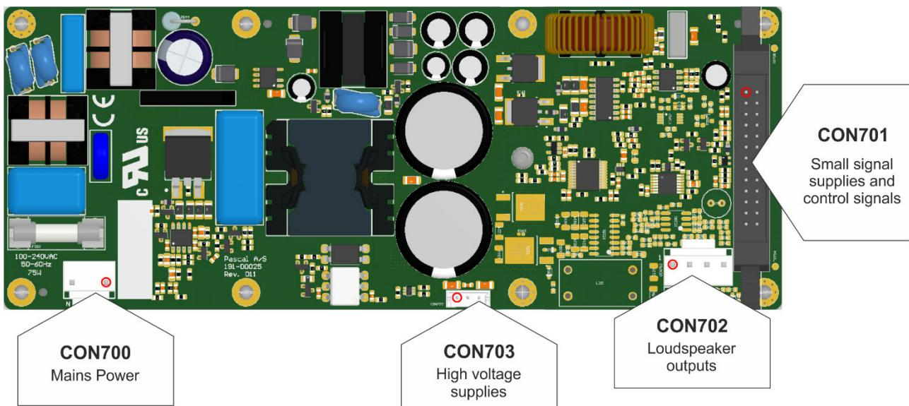
Figure 6-1: U-PRO1 Amplifier module connectors - red circle indicates pin 1
