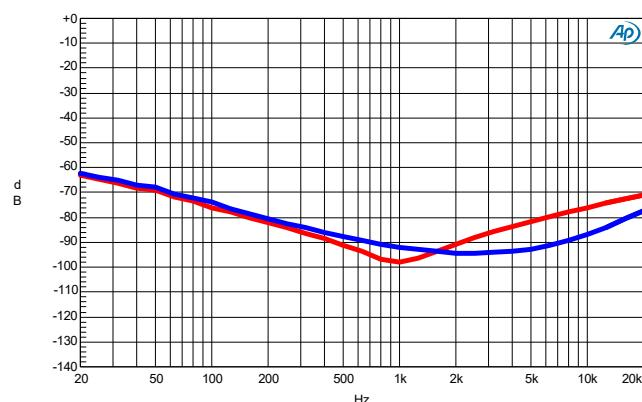
Figure 3-22: Cross talk - Ch.1 @ Po, ch2=50W 8Ω (red), Ch.2 @ Po, ch1=50W 8Ω (blue)
