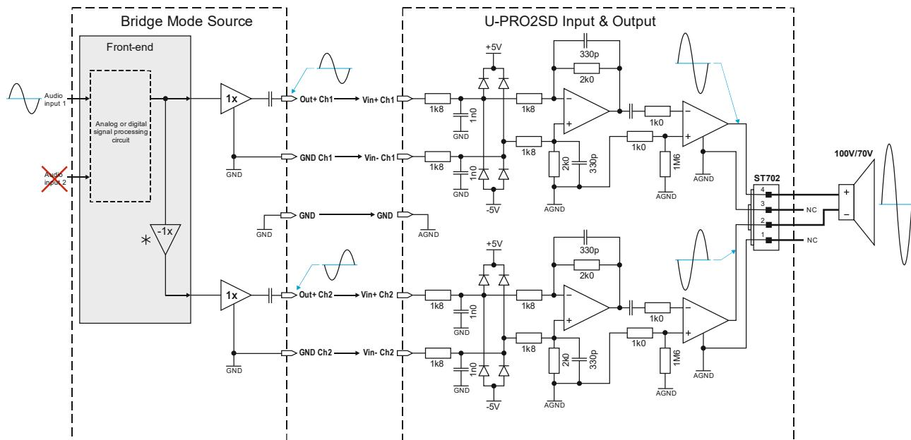
Figure 5-4: U-PRO2SD Amplifier module shown in Bridge Tied Load (BTL) configuration driving one 100V/70V line
