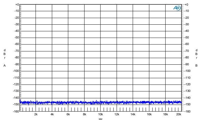
Figure 3-12: FFT idle -  $66\Omega$  BTL
