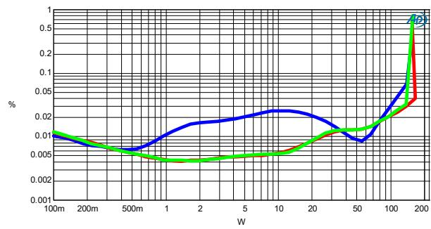
Figure 3-4 THD+N vs. Power @ 8Ω, 230VAC
