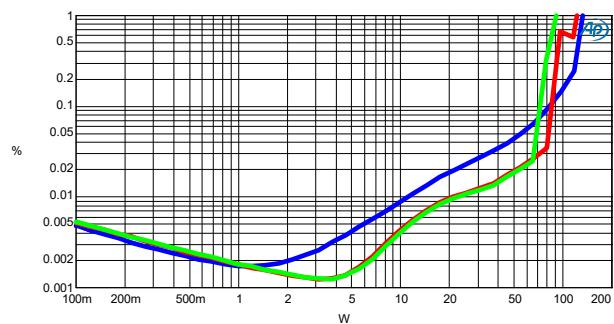
Figure 3-10: THD+N vs. Power @  $66\Omega$ ,  $120V_{AC}$
