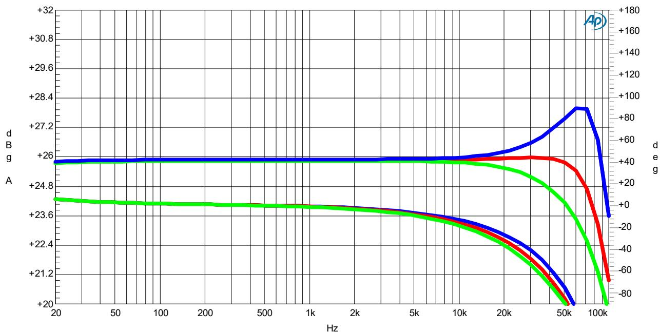
Figure 3-1: Frequency response (Top curves: Amplitude, Bottom curves: Phase)
