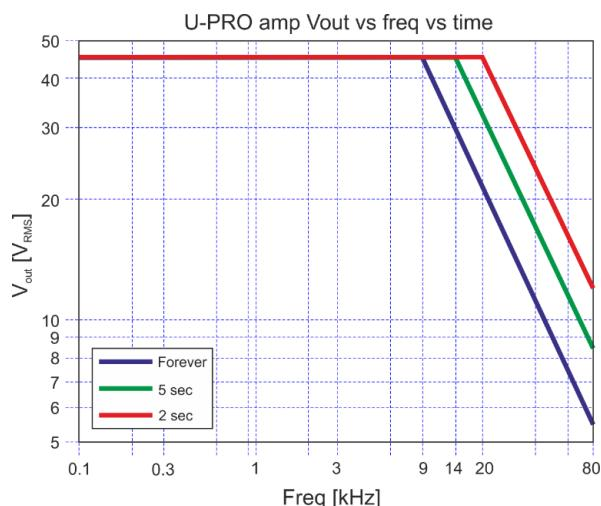
Figure 3-23: Max Vout vs. frequency vs. time
