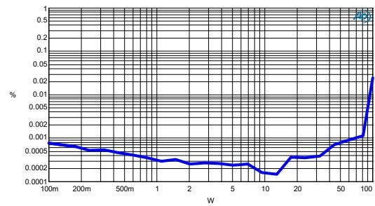
Figure 3-18 CCIF vs. Power -  $R_L=66\Omega$
