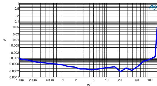
Figure 3-17 CCIF vs. Power -  $R_L=40\Omega$
