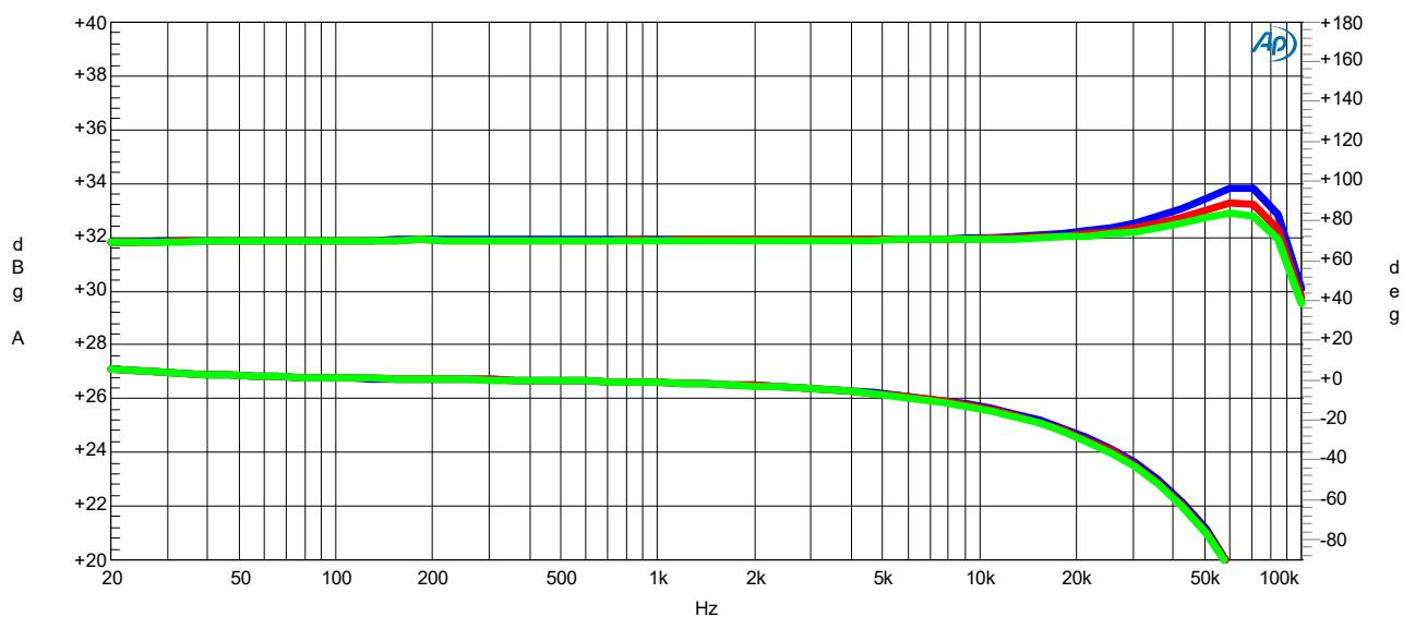
Figure 3-2: Frequency response (op curves: Amplitude, Bottom curves: Phase)
