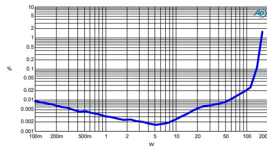
Figure 3-20 TIM vs. Power -  $R_L=66\Omega$ , 230VAC
