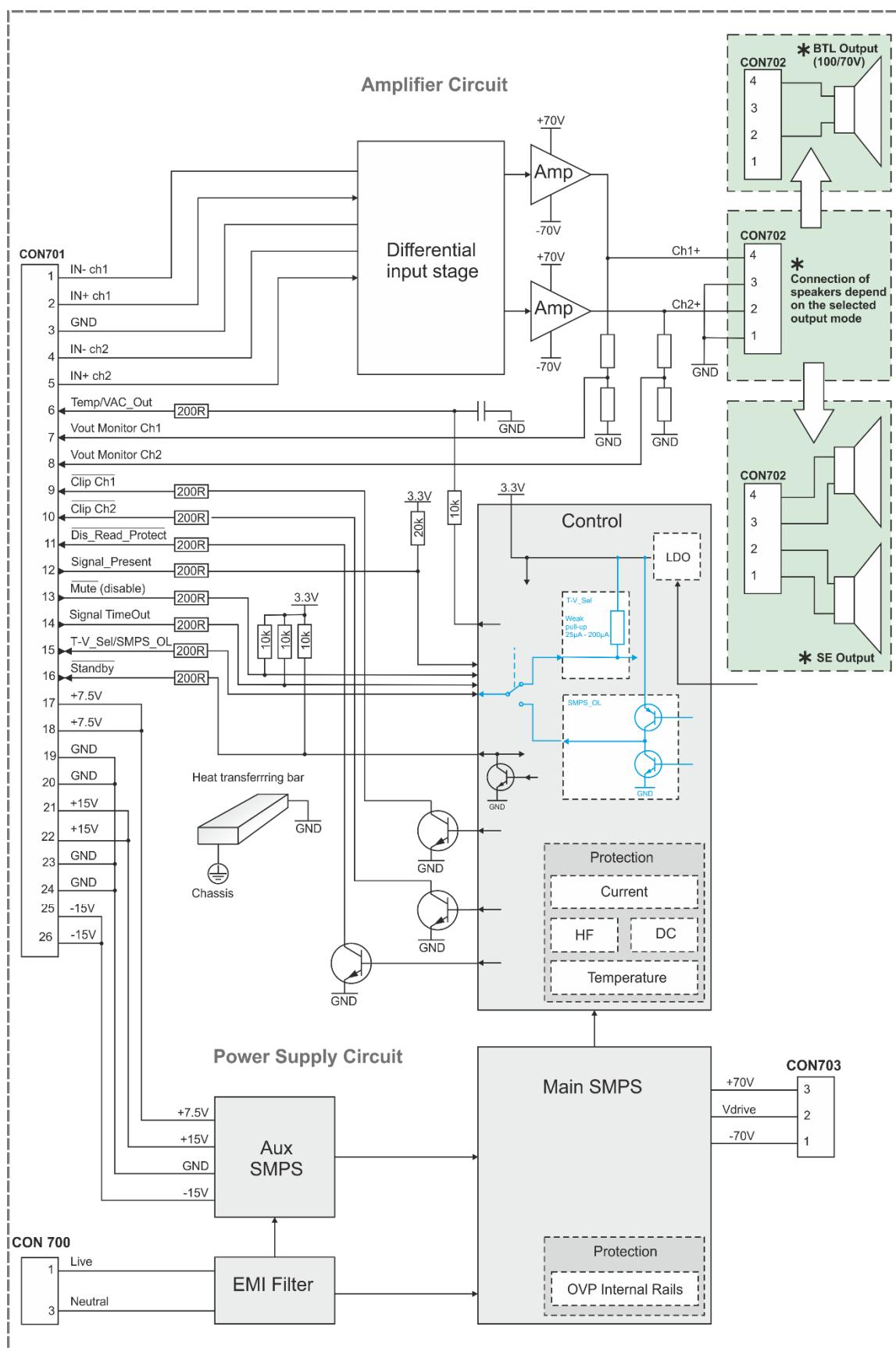
Figure 5-1: Block diagram showing U-PRO2SD module functionality
