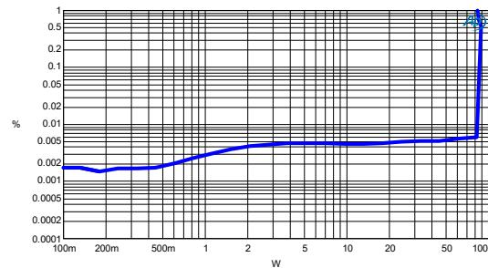
Figure 3-14: CCIF vs. Power -  $R_L=8\Omega$
