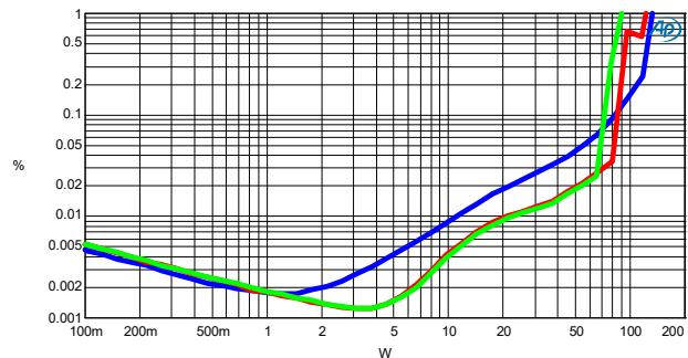
Figure 3-8: THD+N vs. Power @  $66\Omega$ ,  $230V_{AC}$
