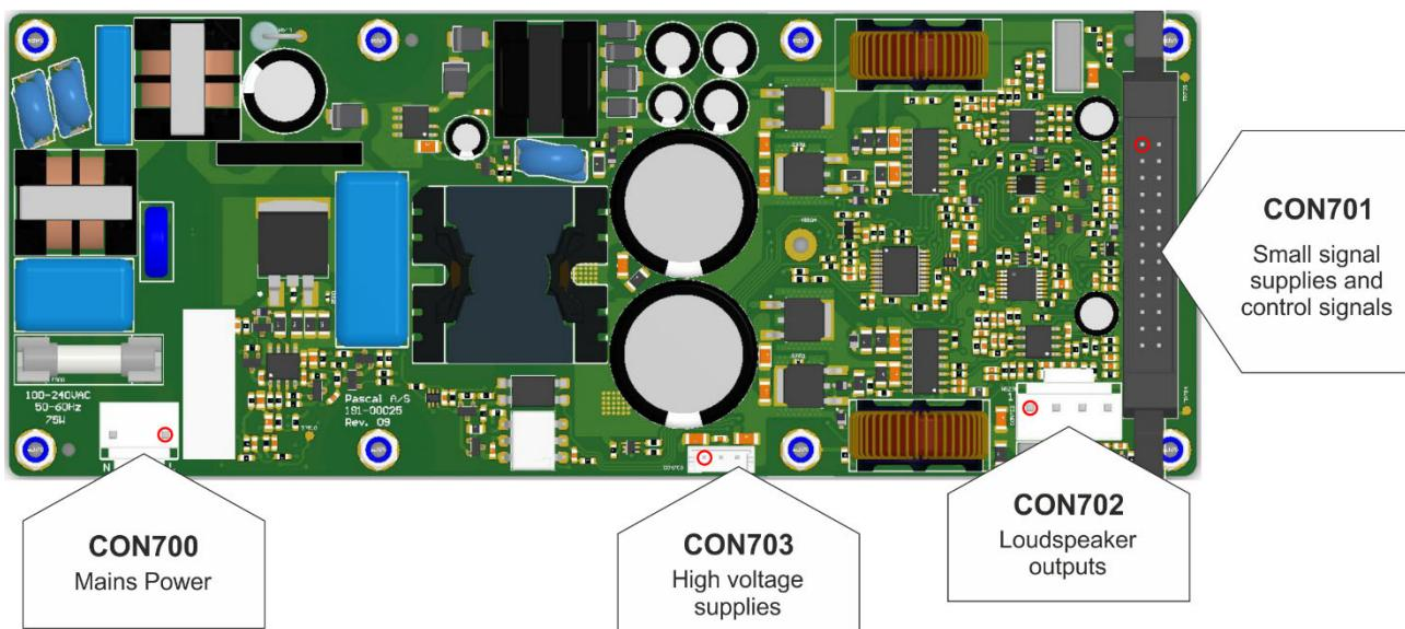
Figure 6-1: U-PRO2SD Amplifier module connectors - red circle indicates pin 1
