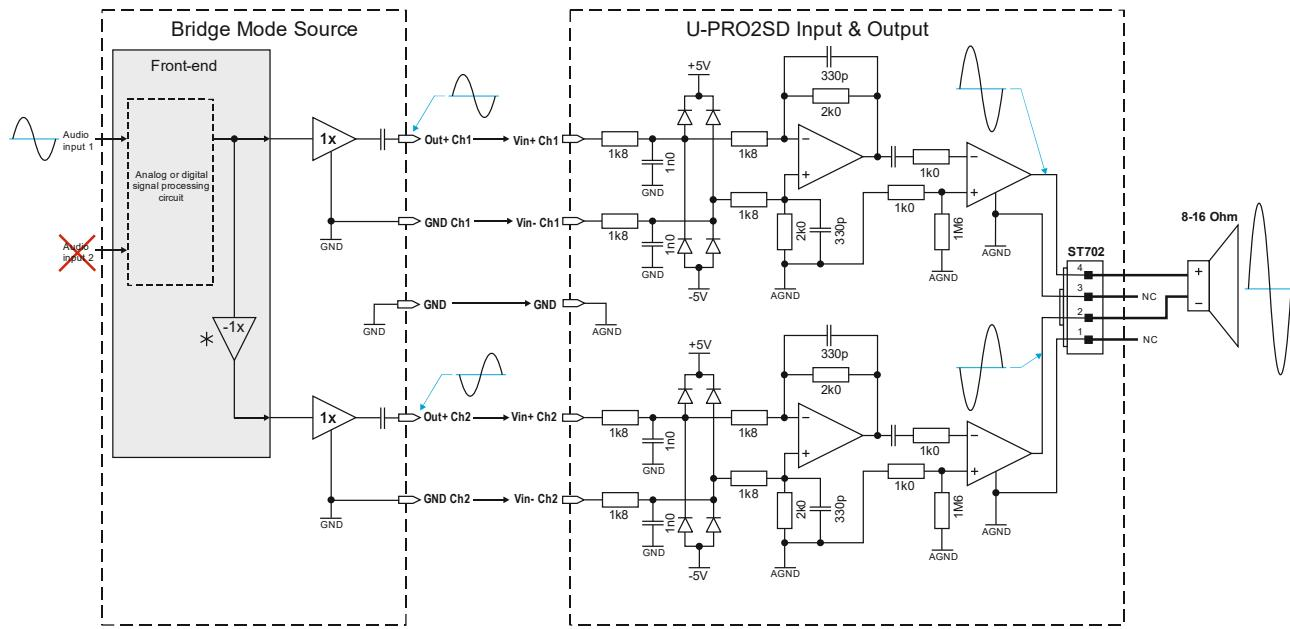
Figure 5-3: U-PRO2SD Amplifier module shown in Bridge Tied Load (BTL) configuration driving one subwoofer
