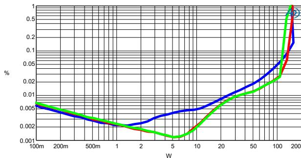
Figure 3-7: THD+N vs. Power@  $40\Omega$ ,  $230V_{AC}$
