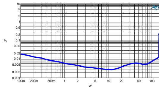
Figure 3-16: TIM vs. Power -  $R_L=8\Omega$ , 230VAC Ch1 (blue)
