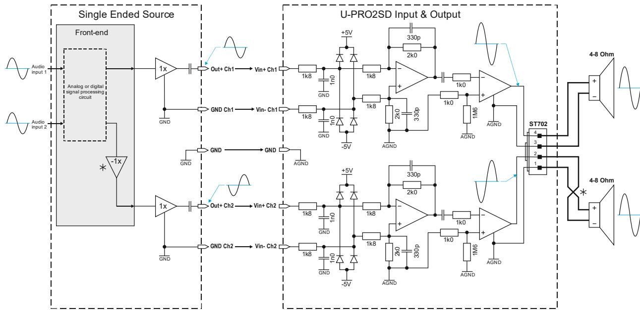
Figure 5-2: U-PRO2SD Amplifier module shown in Single Ended (SE) configuration driving two identical LF/MF loads
