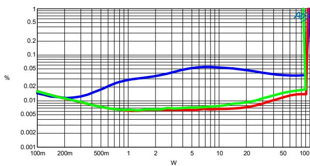
Figure 3-5 THD+N vs. Power @ 4Ω, 120VAC
