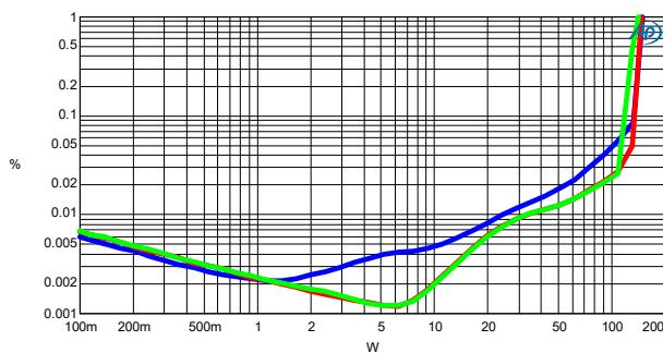
Figure 3-9: THD+N vs. Power@  $40\Omega$ ,  $120V_{AC}$
