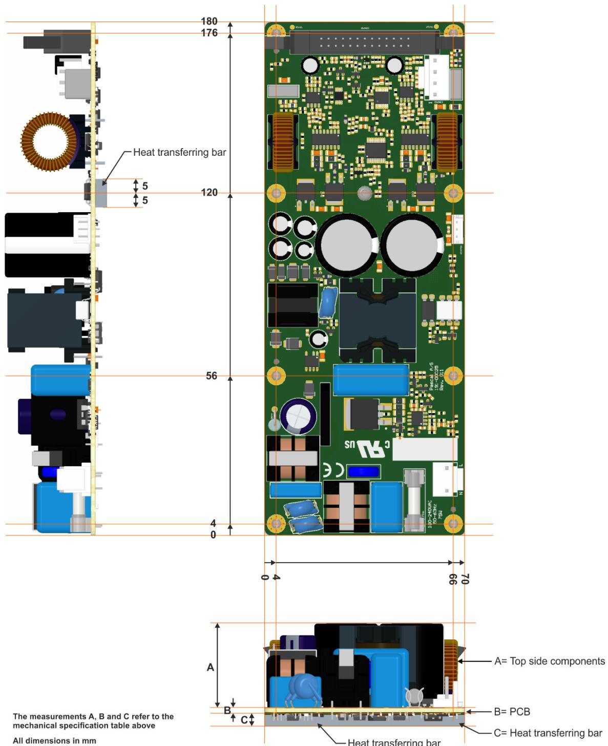
Figure 7-1: Mechanical outline and specifications for the U-PRO2SD module
